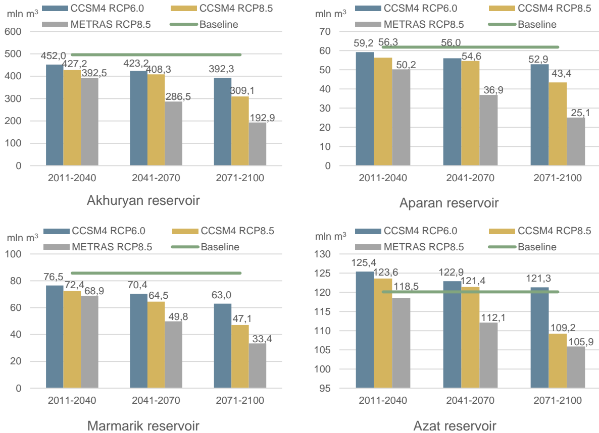
Figure 5-14. Vulnerability of the river inflow during spring floods
